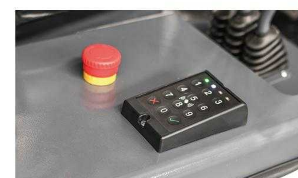
Emergency switch + Pin-code lock
