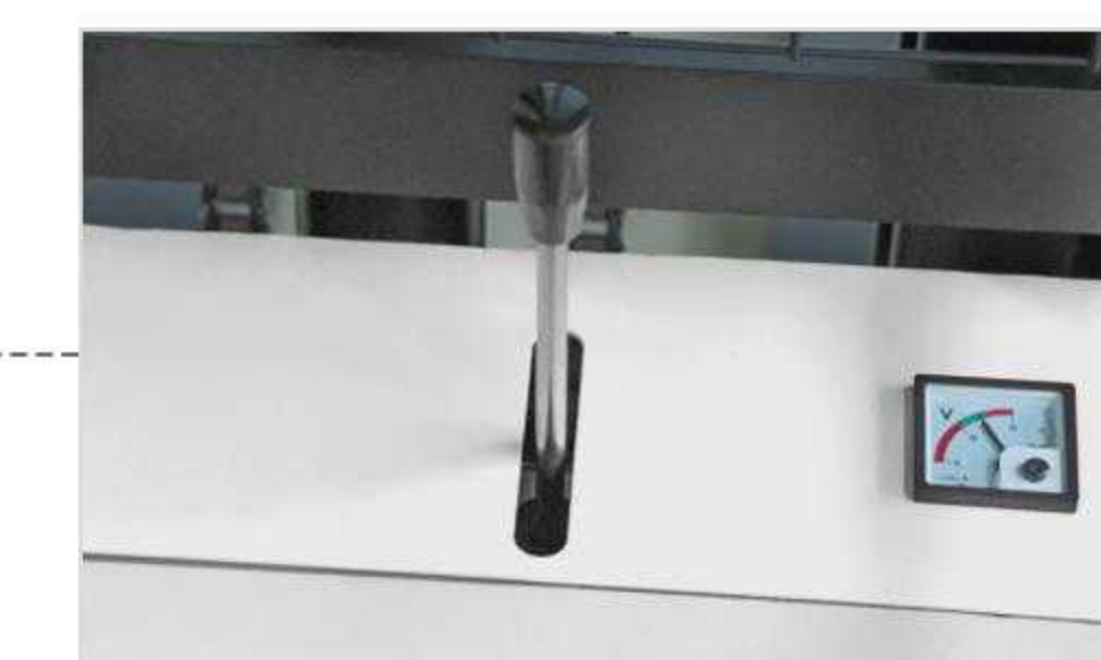
Use handle to control fork height electrically
