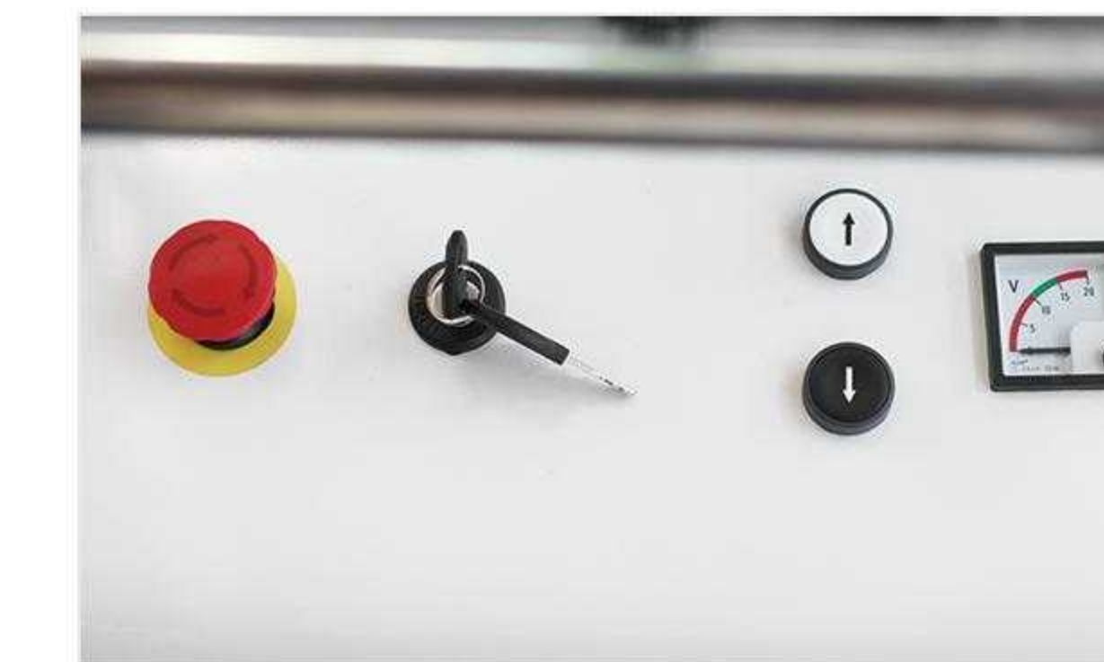
Emergency stop, Key to lock, Lifting and lowering button.
