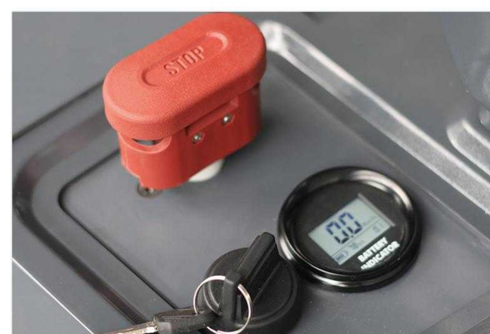
Emergency switch Battery indicator
